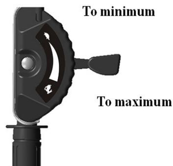
Figure 13 Accelerator valve regulator
